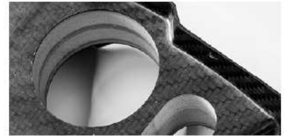
Machining processes compared: dry (left), rhenus special coolant (right)
